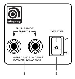
1. 1/4" TS Full Range Input / Output Jacks: The jackplate features two 1/4" jacks wired in parallel, allowing easy daisy-chaining from one speaker cabinet to another. Each of the jacks may be used as an input or a through connection.
