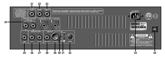
**21. FOOTSWITCH:** Use this jack to connect a two button footswitch for remote Mute and EQ On/Off control. (Tip = Mute, ring = EQ On/Off.) When a footswitch is connected, the Mute switch (#3) remains active; however, the Graphic EQ switch (#12) is disabled.
