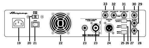
IEC POWER INPUT CONNECTOR: This is where you connect the supplied AC power cord.
