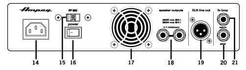
18. SPEAKER OUTPUTS: These 1/4" TS Speaker Output jacks supply speakerlevel power to the speaker cabinet. The rated power output is 250 Watts RMS into  $8 \Omega$ , or 350 Watts RMS into  $4 \Omega$ .
