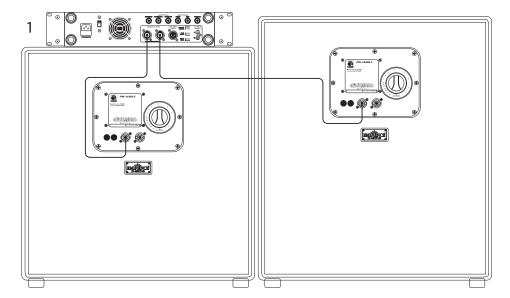
1. A speaker cable with Speakon ends connects from one Speaker Output of the amplifier to the Speaker Input of an Ampeg Pro Neo PN-115HLF cabinet. Additionally, an Ampeg Pro Neo PN-410HLF cabinet is connected from the remaining Speaker Output of the amplifier to the cabinet's Speaker Input using a speaker cable with Speakon ends.
