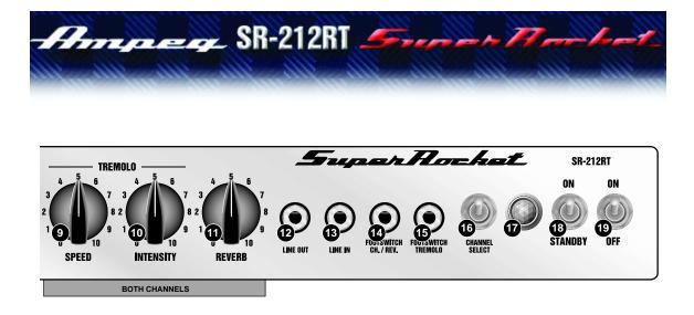
**12. Line Out:** Use this jack to: (1) send a line-level signal to the input of an external effect for additional signal processing, or (2) send a line-level signal to an external amplifier, recording console or mixing board.
