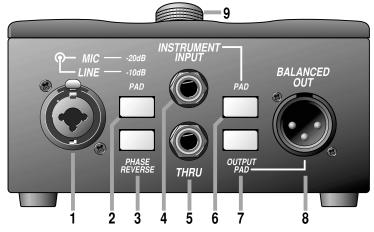
**1. MIC/LINE:** Connect a mic input signal to the balanced XLR jack by means of a high quality shielded cable. This input is designed for mic input sources only. Connect a balanced line signal to the inner 1/4" T/R/S jack. This jack is designed to accept balanced line level signals.
