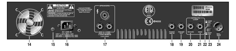
14. (FAN): The temperature controlled, variable speed fan draws cool air into the amplifier and forces heat out through the exhaust vents (also on the rear panel, between the speaker jacks and the power amp in jack). *Do not obstruct the fan or vent hole openings.*
