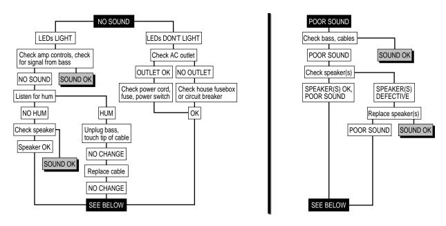
If the problem isn't covered above, or if the steps led you here, then contact your Ampeg dealer for service information. Also, you should refer your amp for servicing if it gets dropped, has liquid spilled into it, or sustains damage to its power cord.
