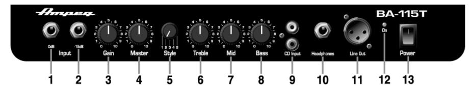
**1. 0dB INPUT:** Connect your "passive" bass guitar here using a shielded instrument cable. This input is not padded and is best suited for basses without active electronics or "hot" pickups.
